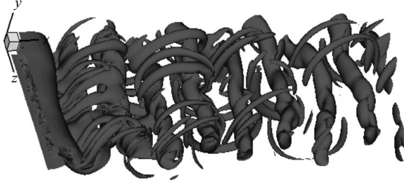
FIGURE 1. Isocontour of the instantaneous vorticity, \Omega/\Omega_{max} = 0.1 .
